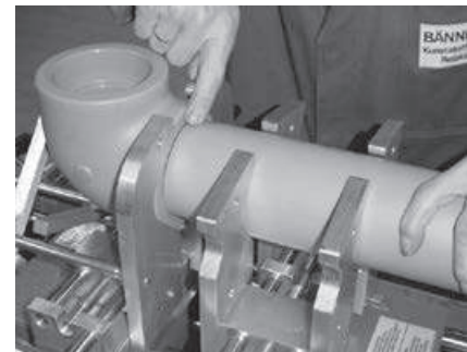
Fig. 8 Lay the pipe axially into the fitting and place in such a way that it is situated frontally to the fitting
