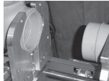
Fig. 10 After the warming time join pipe and fitting
